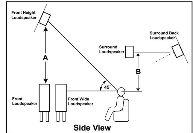
Both the Front Height and Surround Back Loudspeakers should be pointed slightly downward. Dolby recommends the **A** dimension be at least 3.3ft (1m). The **B** dimension should be between 2-3ft (60-90 cm). Before starting Audyssey Auto Setup, place the setup microphone in the main listening position. Audyssey MultEQ® XT uses the measurements from this position to calculate speaker distance, level, polarity, and the optimum crossover value.
